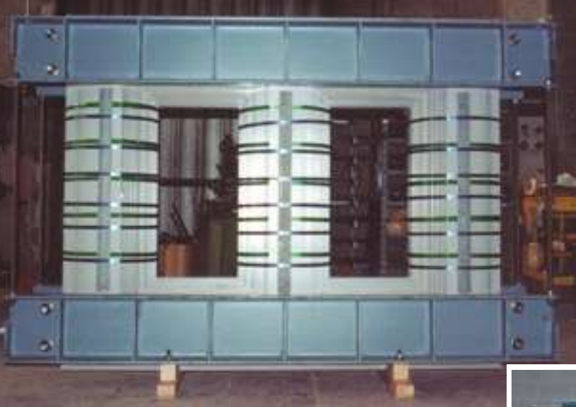
20 MVA - NUCLEO MAGNETICO - MAGNETIC CORE
